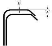
SELF DRILLING FASTENERS MUST DRILL THROUGH BOTH PURLINS BEFORE ENGAGING THREADS IN TOP PURLIN....
