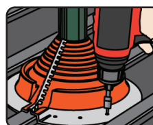
5. Fasten Retrofit to roof
